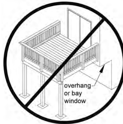
Figure 18. No Attachment to House Overhang with Ledger.
